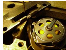
Bobbin case indexing-vertical axis
